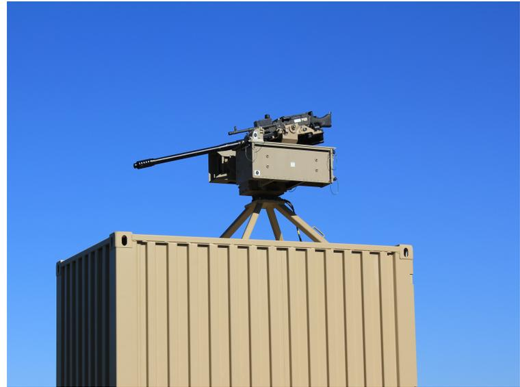
The lifting mechanism/platform can accommodate **5,000** pounds of payload . The retractable roof panel affords enough clearance to allow the deployment of the XM914/M230LF 30mm 30x113 cannon. Operations can be conducted both with and without the trailer. The stiffness of the container, paired with the R400S Mk2's stabilization affords unequalled accuracy and precision for any weapon combination.
