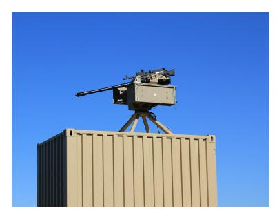
The lifting mechanism/platform can accommodate **5,000** pounds of payload . The retractable roof panel affords enough clearance to allow the deployment of the XM914/M230LF 30mm 30x113 cannon. Operations can be conducted both with and without the trailer. The stiffness of the container, paired with the R400S Mk2's stabilization affords unequaled accuracy and precision for any weapon combination.
