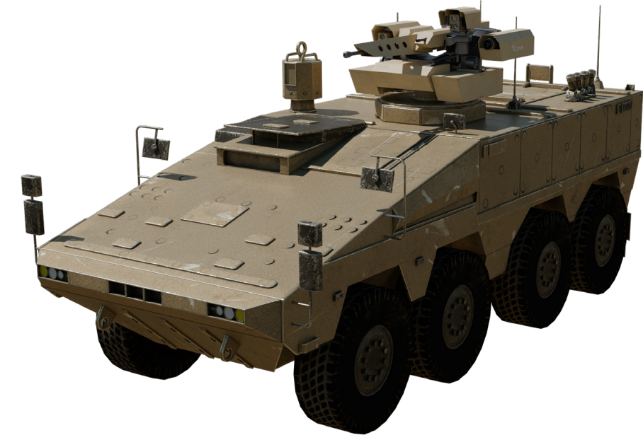
R800 on Boxer with new Stanag level 3 armour design
